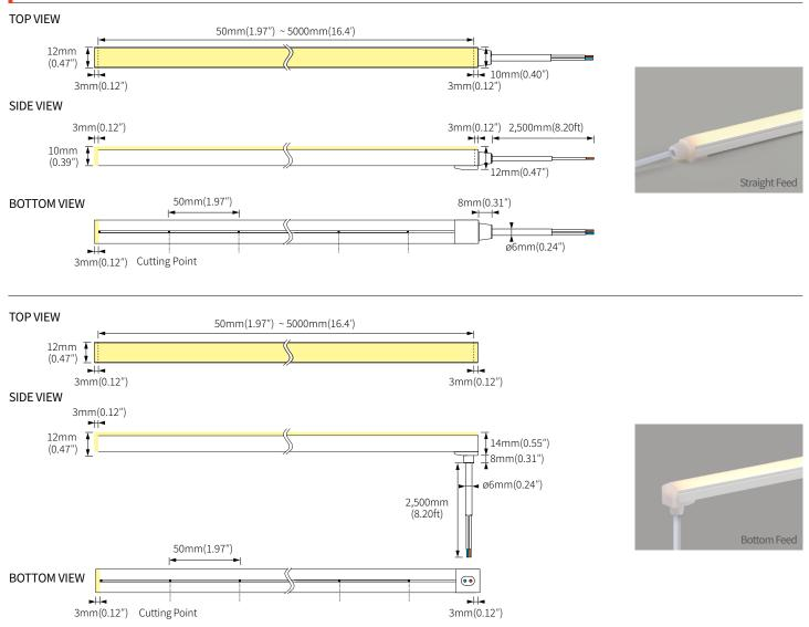
FLXible Neon can be cut every 50mm (1.97"). Please follow the cutting point mark to cut precisely as needed.
